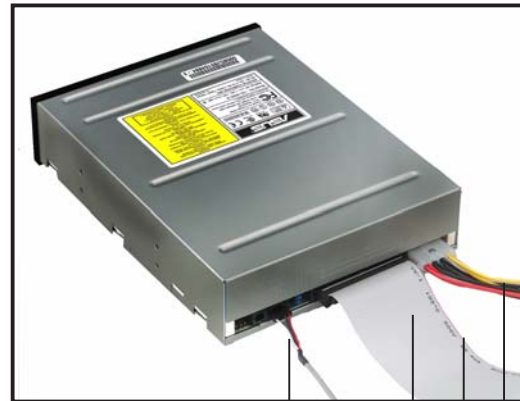
Audio cable IDE ribbon cable Red stripe to pin 1 Power cable
